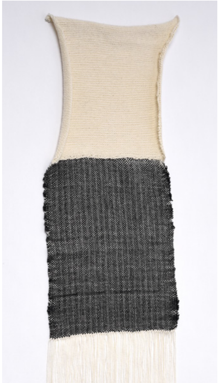
Fig. 55: Sample illustrating the seamless combination of a knitted surface (above) with a woven one (below)
