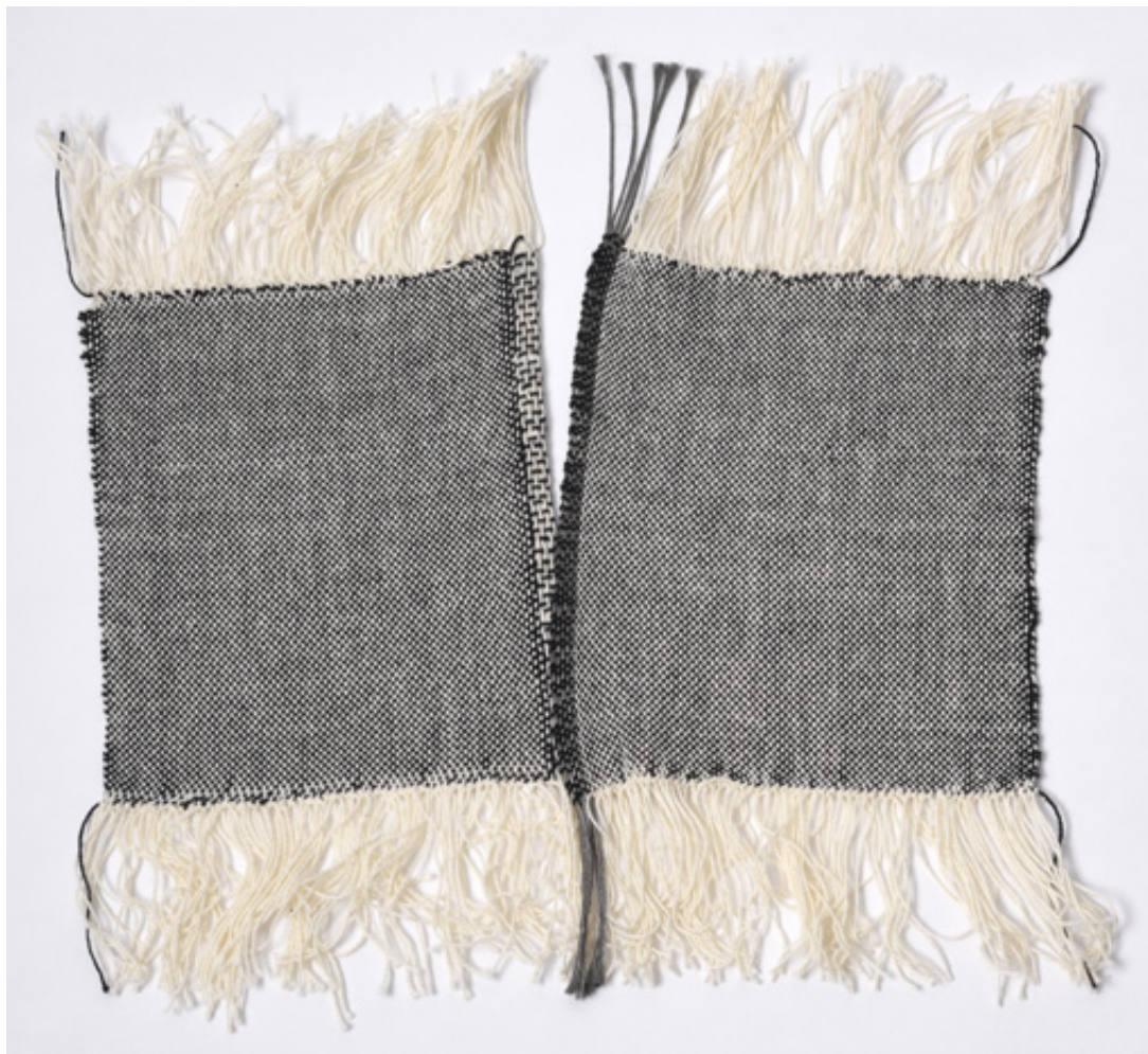
Fig. 59: Attachment system using magnetic yarns woven into the edge of the fabric
